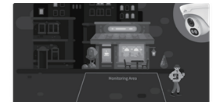
Events end (human/vehicle leaves) IR on, warm light off
